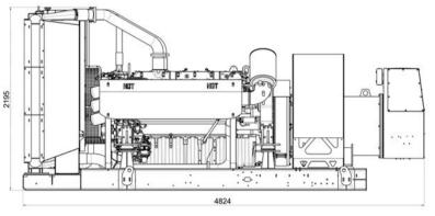
Drawing above for illustration purposes only, based an standard open power 400 Volt engine-generator set. Lengths may vary with other voltages. Do not use for installation design. See website for unit specific template drawings.
