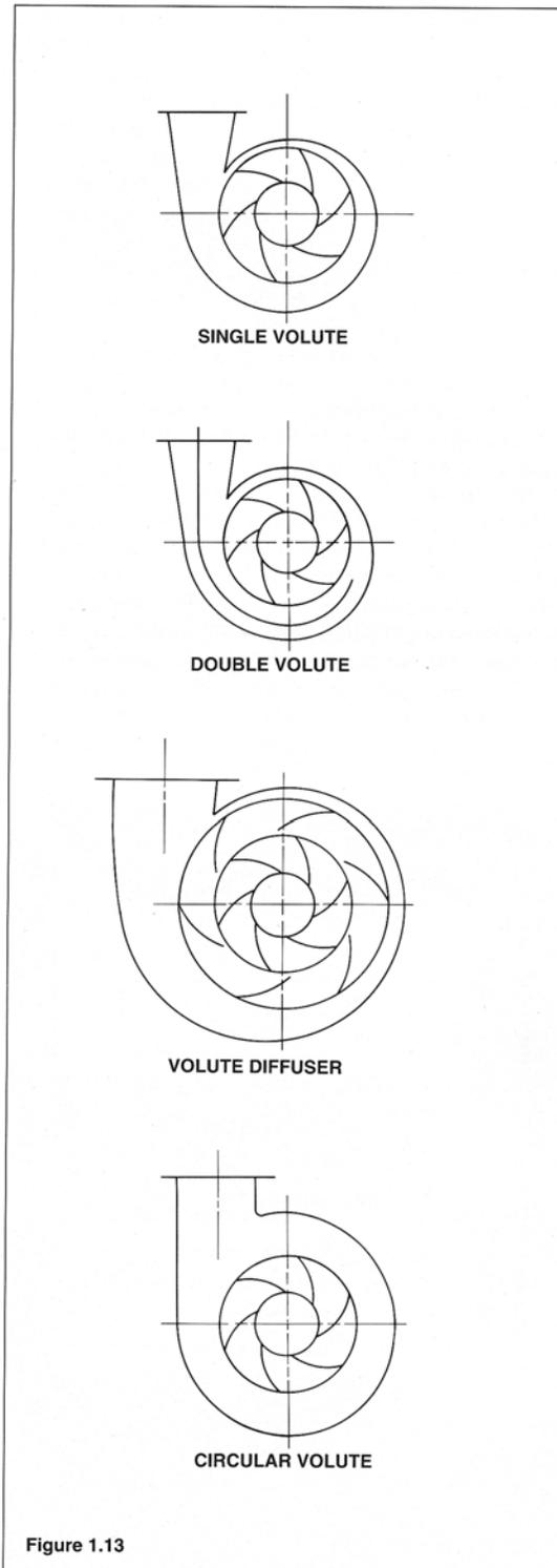
The hydraulic loads are dependent on the type and size of impeller and casing, the pump operating conditions such as fluid suction pressure, and the point of pump operation. The magnitude and direction of the hydraulic loads can change greatly with changes in these factors. In most instances, the lowest hydraulic loads exist only at pump operation at the BEP. Pump cavitation influences operation and consequently the pump hydraulic loads.
