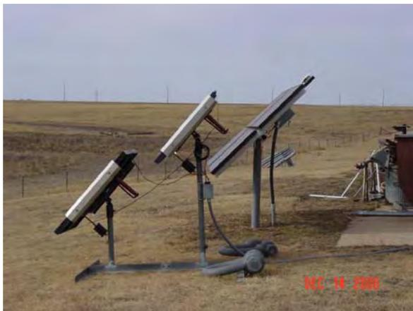
Fig. 7. PV Array tilt angle in fall and winter at Bushland, TX.
