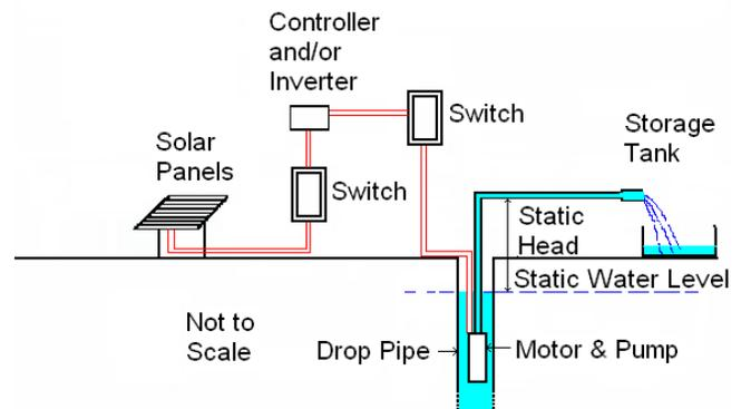
Fig. 1. Schematic of Solar-PV Water Pumping System.
