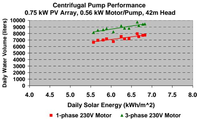
Fig. 19. Effect of AC Motor Phase on Daily Water Volume of Solar Powered Centrifugal Pump System.
