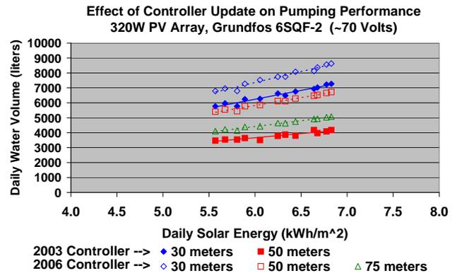
Fig. 13. Effect of Controller Update on Solar Powered Helical Pump System (320W PV).
