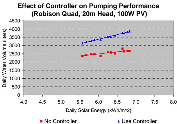
Fig. 12. Affect of Use of Controller on Daily Water Volume of a Solar Powered Diaphragm Pump.
