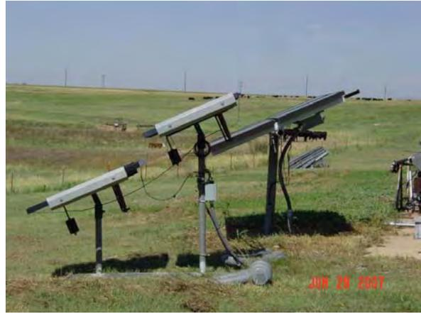
Fig. 8. PV Array tilt angle in spring and summer at Bushland, TX.
