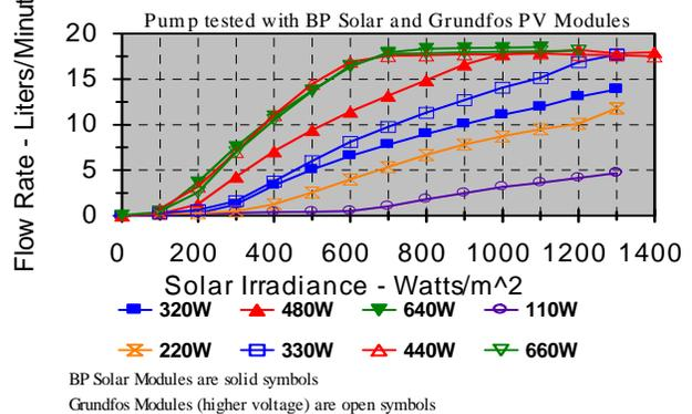
Fig. 10. Affect on Flow Rate of Same Type of Modules but at Different Voltage Ratings.
