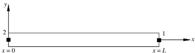
Fig. 1. Uniform Timoshenko beam with free end conditions.
