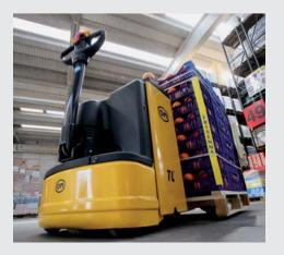
**Pedestrian low lift power pallet trucks TL and TN.** The model range includes the TL for standard and the TN for heavy-duty applications with capacities from 1.600 up to 3.000 kg.
