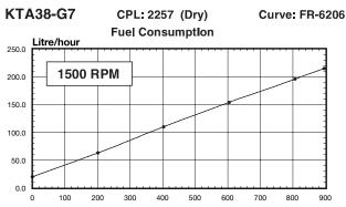
Gross Engine Power Output - kWm (U.S. Gal = Litres x 0.2642) (BHP = kWm x 1.34)
