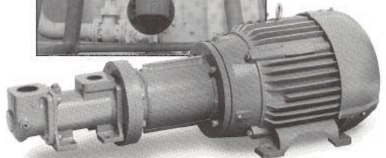
Model A3D with 15 hp magnetic drive and TEFC motor, 15 gpm, 300 psig discharge, 9600 SSU, 1200 rpm. Horizontal foot mounted.
