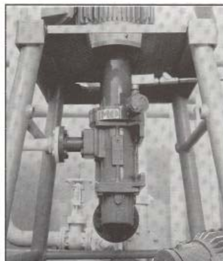
Model MANBC03DVC250SC with 25 hp magnetic drive and TEFC motor, 100 gpm, 210 psig discharge, 190-2400 SSU, 1800 rpm. Vertically face mounted.
