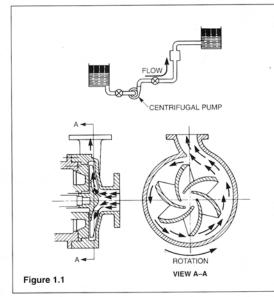
pressure is lowest. This fluid passes through the impeller as still more fluid enters the impeller.
