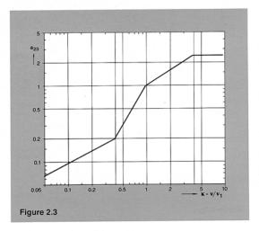
cant viscosity ( $\nu$ ) at the operating conditions to the minimum required lubricant viscosity ( $\nu_1$ ) at the operating conditions. The Kappa value should ideally be greater than 1.5.
