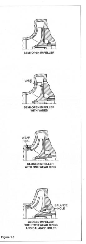
are illustrated in fig. 1.8. The semi-open impeller with pump-out vanes and the closed impeller with two wear rings and balance holes are most common in petrochemical and paper mill process applications.
