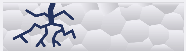
Fig. 1.6.10: Stress corrosion cracking
