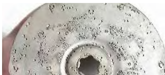
Pitting corrosion of EN 1.4401 (AISI 316)
