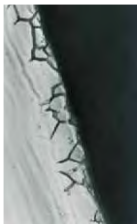
Intergranular corrosion of stainless steel
