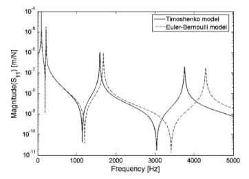
Fig. 9. Point FRF at the spindle tip (the holder and tool are not connected).
