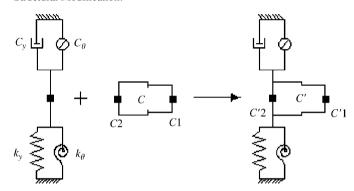
Fig. 4. Receptance coupling of two segments and addition of bearing dynamics to the system by structural modification.
