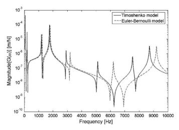
Fig. 12. Tool point FRF for highly stiff connection at spindle–holder and holder–tool interfaces.
