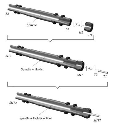
Fig. 6. Elastic coupling of spindle, holder and tool (sectional view).
