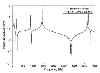
Fig. 11. Tool point FRF for the example case (material loss factor is taken as close to zero).
