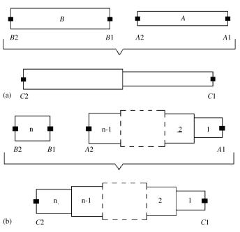
Fig. 2. (a) Rigid coupling of two uniform beams with free end conditions and (b) rigid coupling of the *n*-th segment.
