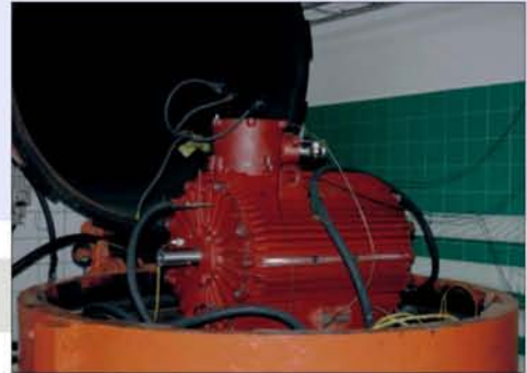
Motor ExSgm 315 M2C 260kW, 1000V, 3000 rpm tested in KD "BARBARA"
